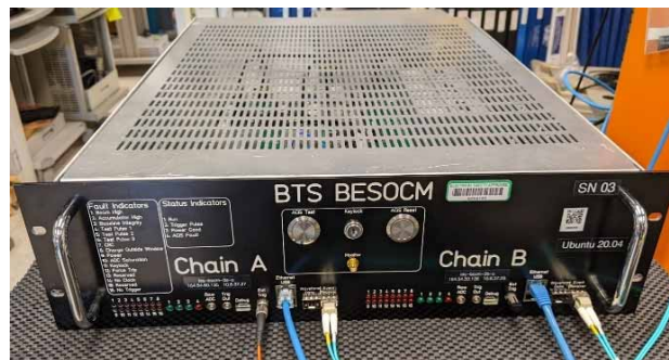
Figure 2: BESOCM chassis, front view.
