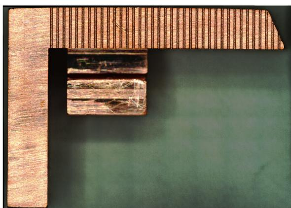
Figure 3: Copper test piece showing 1-mm-spaced rulings on the gap side.
