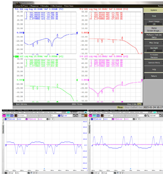
Figure 6: An example of frequency response (upper, A to sum port) and the time domain response (lower left, A to X, lower left A to Y).
