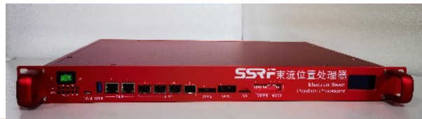
SSRF/SXFEL/DCLS SoC Processor Fs=125MHz, BW=650MHz
