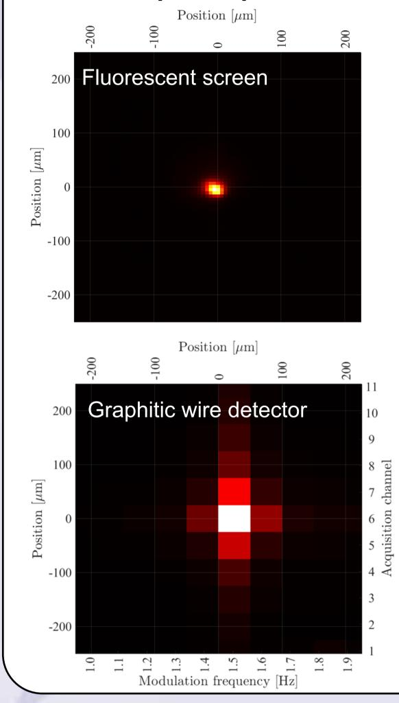
On the I18 beamline at Diamond light Source the X-ray beam was focused down to 20µm x 24µm FWHM in size - much smaller than the 50µm x 50µm pixel pitch of the graphitic wire detector.
