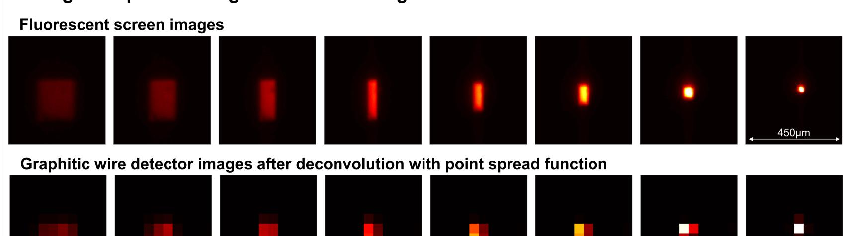
This image sequence was obtained as the beam was focused down at the sample point. The graphitic wire detector can resolve the beam size, shape, and intensity during this operation. Though the resolution is poorer than the fluorescent screen, it is transparent enough to remain permanently in the beam path.
