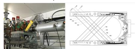
Figure 4: Left: The single WSM on FETS beam line. Right: The monitor head with CNTs. The horizontal wires are upstream of the vertical wires, which are 3 mm apart in the beam direction. The  $\phi 10 \mu\text{m}$  CNT was too thin to be mounted on the monitor head.
