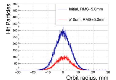
Figure 10: The computed beam profile measured by  $\phi 10 \mu\text{m}$  wire. The initial beam is a Gaussian distribution with the design value of beam size ( $\sigma=5$  mm). The scattering angle and energy loss at the wire are computed by PHITS, which are taken into account in this simulation.
