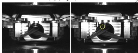
Figure 5: Light emission from the  $\phi 50 \mu\text{m}$  (left) and the  $\phi 20 \mu\text{m}$  (right, in the circle) CNTs with the 3 MeV FETS H-beam. The wire was aligned at the centre of the beam pipe when the photo was taken.
