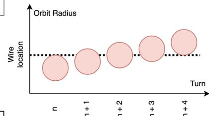
Figure 1: Schematic drawing of the profile measurement of an accelerating beam over several turns (red circles) in the FETS-FFA ring.
