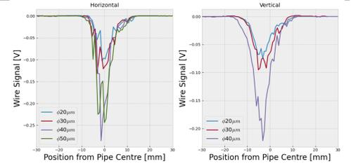
Figure 7: Beam profiles measured by each CNT wire. The scan range was 148.5 mm with a step size of 1 mm. The peak pulse intensity measured by the CT monitor was about 13 mA in this measurement.
