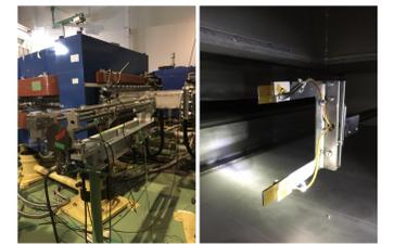
Figure 8: The radial probe (left) and the monitor head of the single WSM with  $\phi 10 \mu\text{m}$  CNT wire (right). The monitor head was attached on the radial probe controlled by the motion control driver.
