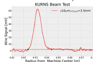
Figure 9: The accelerating multi-turn beam profile measured by  $\phi 10 \mu\text{m}$  CNT wire. The dashed line is the 2 times of standard deviation of the noise level, computed by the RMS within a time window at the end of the data when there is no beam.
