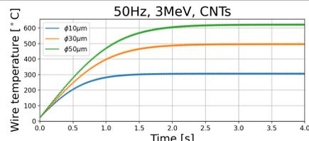
Figure 3: Transient temperature in each CNT wire. A thermal emissivity of CNT in vacuum is estimated to be 0.2 in this simulation.
