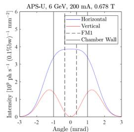
Fig. 2: Vertical profile of bending magnet synchrotron radiation accepted by 35-BM for APS-U storage ring. The vacuum chamber wall blocks synchrotron radiation at angles  $\pm 1.0$  mrad. The first fixed mask (FMI) blocks synchrotron radiation at angles  $> \pm 0.35$  mrad.
