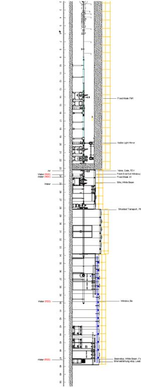
Fig. 7: Illustration of 35-BM beamline profile for APS-U operations. The horizontal axis  $z$  is the distance from the bending magnet source in metres. The beam direction in this figure is from top to bottom.
