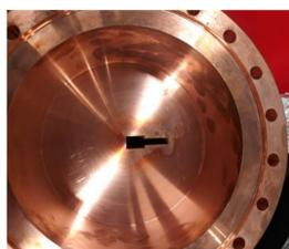
Fig. 4: Machining of FM1 vertical aperture to increase the vertical aperture for visible light propagation. The narrower slot (at right) is used to pass X-rays through to the X-ray beamline enclosures. The beam direction in this figure is into the page.
