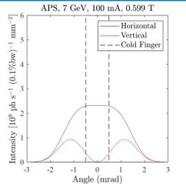
Fig. 1: Vertical profile of bending magnet synchrotron radiation accepted by 35-BM for APS-U storage ring. The cold finger masks synchrotron radiation over the central  $\pm 0.5$  mrad.
