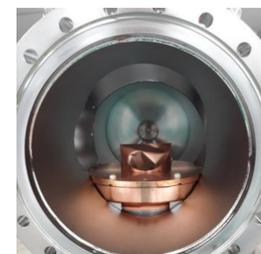
Fig. 5: Visible light mirror. The beam direction in this figure is into the page.
