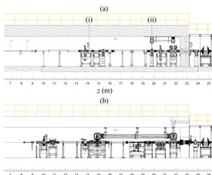
Fig. 3: Comparison of 35-BM front ends for APS-U and APS. The horizontal axis  $z$  is the distance from the bending magnet source in metres. (a) Front end configuration for APS-U. (i) First Fixed Mask. (ii) Visible Light Mirror. (b) Front end configuration for APS.
