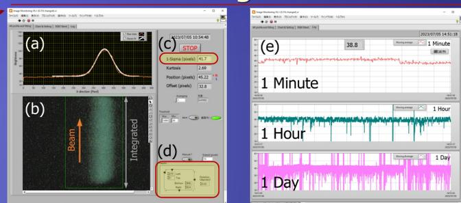
(a) Result of integrating the brightness and a Gaussian fit  $1\sigma$
