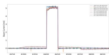
A low current beam pulse measured by 8 BCMs from the LEBT to the DTL4
