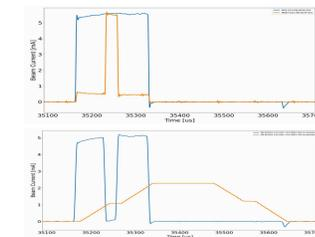
Absolute (above) and differential (below) beams with the RFQ-MEBT1 differential pair
