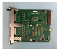
LVDS to RS485/optical converter AMC
