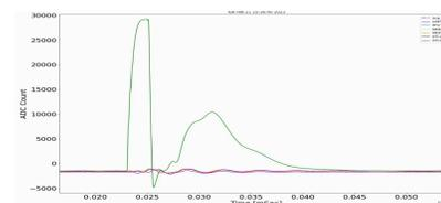
An RF breakdown in the DTL2 causing ringing with the other BCMs (with cal. windings being connected)
