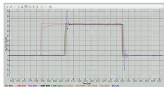
A high current beam pulse measured by 9 BCMs from the ISrc to the DTL4, and a FC at the end of DTL4.
