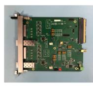
LVDS to RS485/optical converter AMC
