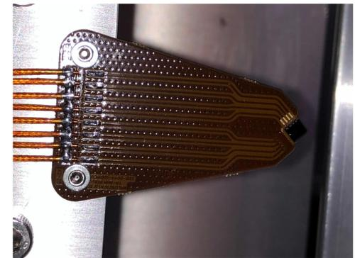
A printed circuit connects the 8 electrodes on the diamond (right) to 8 coaxial cables that run to a nearby amplifier box covered in shielding.
