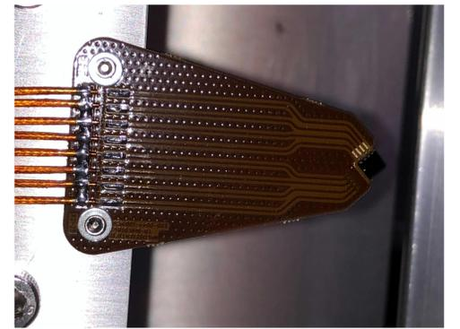
A printed circuit connects the 8 electrodes on the diamond (right) to 8 coaxial cables that run to a nearby amplifier box covered in shielding.
