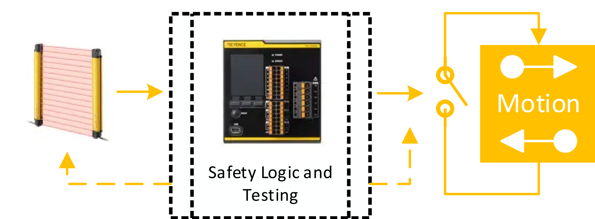
Figure 5: Light Barrier Safety Design (PLe rating)
