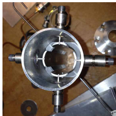
Figure 6: Electrostatic deflector showing the curved plates.
