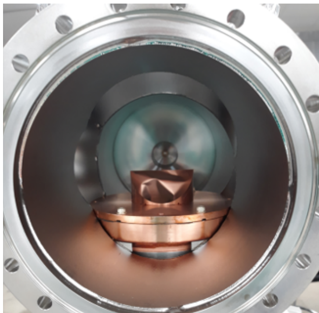
Figure 5: Visible light mirror. The beam direction in this figure is into the page.
