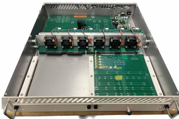
Figure 3: Mockup of common platform chassis with carrier module and one of two daughter cards installed.
