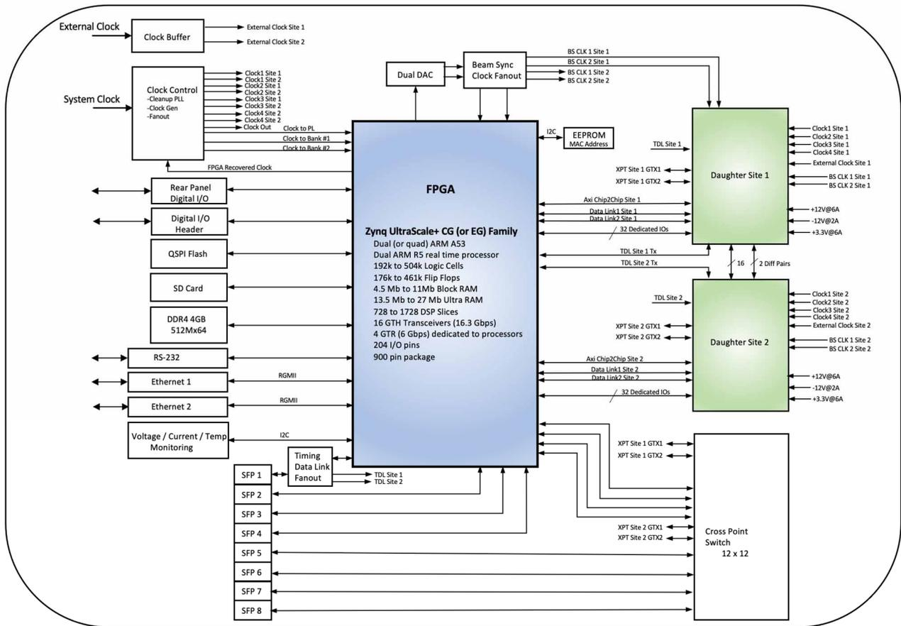
Figure 4: Block diagram of common platform carrier board.
