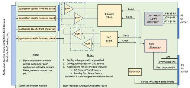
Figure 7: Block diagram of precision ADC/DAC daughter card.
