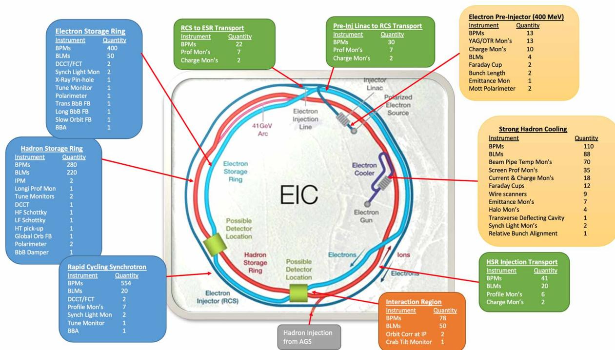
Figure 2: EIC instrumentation list for each subsystem, excluding the existing hadron injector machines.
