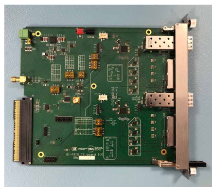
Figure 6: Photo of the new LVDS to RS-485/optical converter AMC (Courtesy of Pawel. K. Jatzak - WUT).
