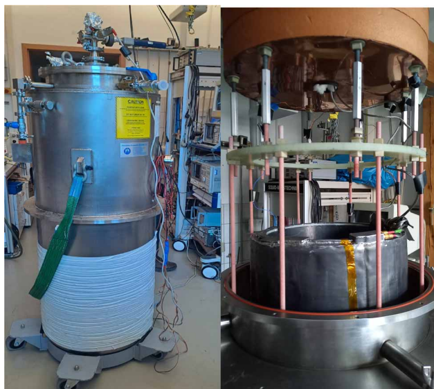
Figure 4: Left: FSU Jena Laboratory with wide-neck cryostat. Right: Axial coreless CCC during installation, the squid box and the cabling is also visible on the top of the CCC. The white windings on the cryostat are the Helmholtz coils for the magnetic shield test. The CCC is at rest in the bottom part of the cryostat.
