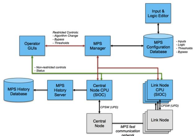
Figure 5: The MPS software architecture.
