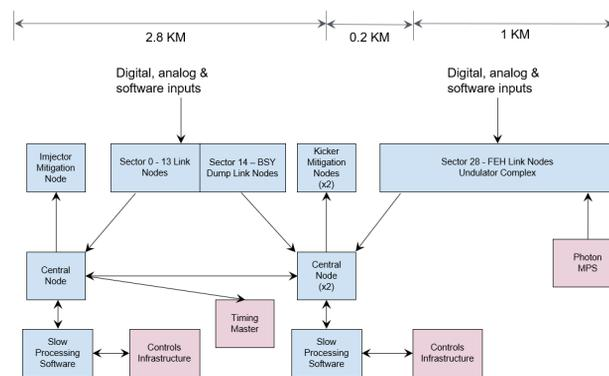
Figure 4: The overall design of the LCLS-II MPS system.
