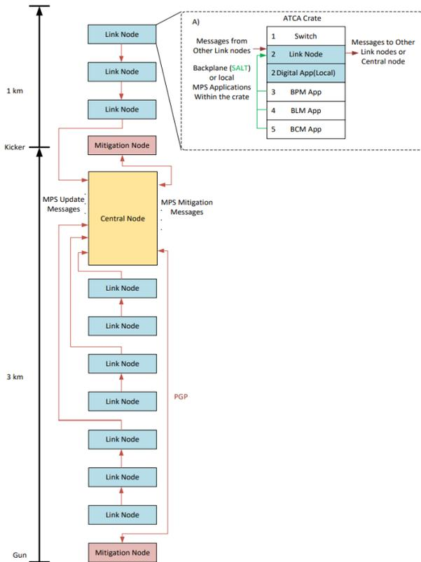
Figure 2: The low-latency MPS communication network.
