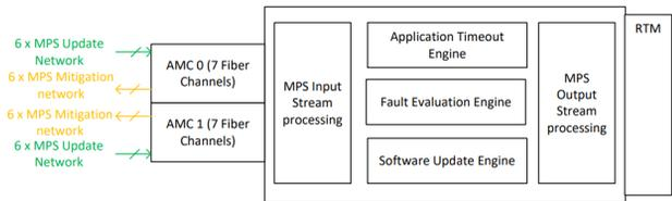
Figure 3: The high-level central node architecture.
