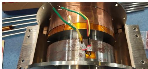
Figure 10: A bypass capacitor over the ceramic gap was built in the APEP-CT sensor.
