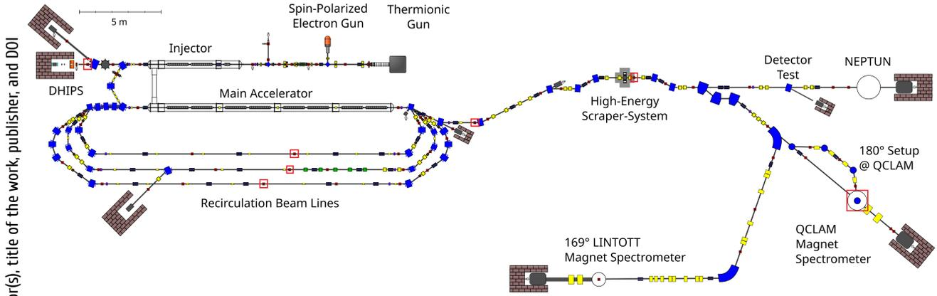
Figure 1: Floorplan of the S-DALINAC. The electrofission experiment as well as the beam stabilization system will be set up at the QCLAM spectrometer. The OTR setups marked in red will be upgraded with fast cameras to allow high-precision beam stability measurements.
