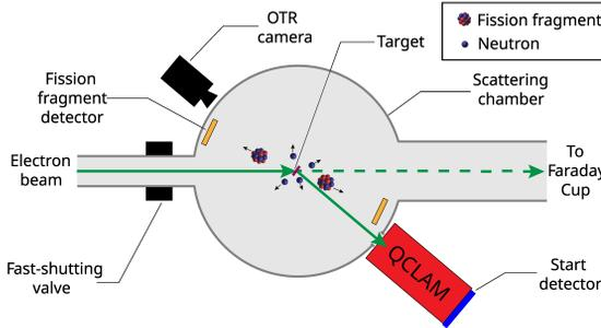
Figure 2: Schematic overview of the electrofission setup design. After interacting with an electron the target nucleus decays via fission. Both fission fragments are detected in coincidence with double sided silicon strip detectors.
