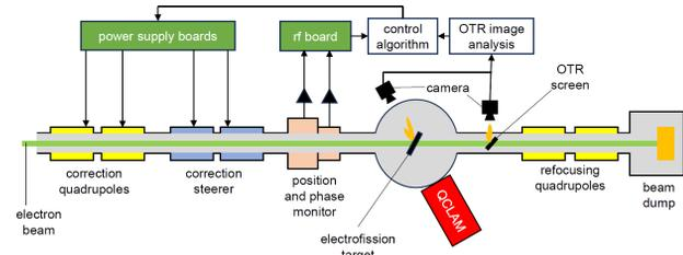
Figure 3: Sketch of the beam stabilisation system. OTR light emitted by both the electrofission target and OTR target is evaluated to determine the beam profile. Additionally, a non-destructive beam position measurement is deduced with a resonator cavity. The signal will be processed by the control algorithm to adjust the correction magnet currents.
