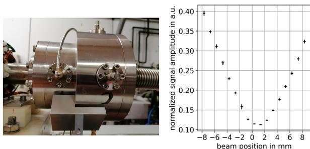
Figure 4: Left: Image of an in-house developed cavity beam position monitor for non-destructive phase and beam position measurements. Right: Test of a decommissioned cavity beam position monitor with existing readout electronics at a beam current of 500 nA. Beam positions with an increment of 1 mm can be resolved.
