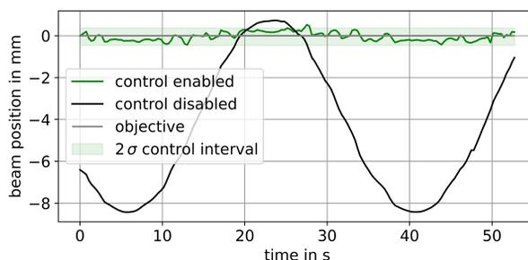
Figure 5: First test of a beam stabilization with a PID controller and implemented fast target analysis algorithm. Despite the strong simulated distortion, the correction magnet was able to keep the center beam position within a  $2\sigma$ -interval of 0.84 mm.
