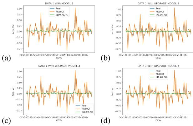
Figure 3: The blue line represents the actual data for 96 OCs obtained through the SVD algorithm. The orange line represents the predicted values for the same OCs obtained through NN models. The green line shows the difference between the actual and predicted values. The green value corresponds to the total error (AE) calculated across all 96 OCs. The horizontal axis shows the 96 orbit correctors. (a) The first model, (b) the first upgrade, (c) the 2nd modification, (d) the 3rd upgrade.
