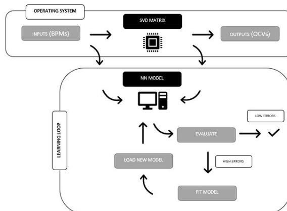
Figure 1: The BPM and OCV datasets from the real system are fed into the learning loops. The NN model uses the BPMs to generate new OCVs, and the error between the predicted and real OCVs is calculated. If the error exceeds the expected threshold, the NN model is updated with the current dataset and replaces the old NN model. This loop is repeated periodically to refine the NN model.
