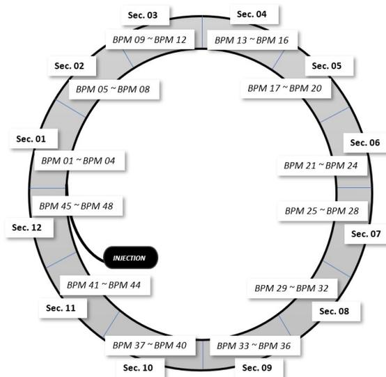
Figure 2: schematic of the CLS (Canadian Light Source) storage ring that comprises twelve sections and 48 BPMs.
