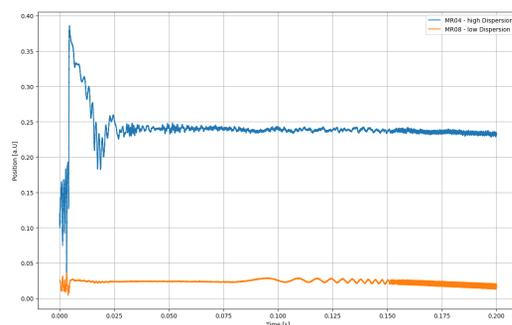
Figure 1: Qualitative position measurement in high and low dispersion regions of the synchrotron.
