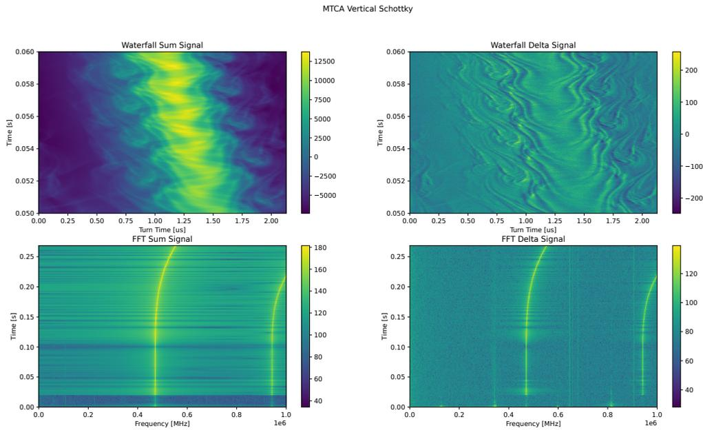
Figure 3: Waterfall diagram and frequency analysis of beam injection with the Vadatech  $\mu$ TCA solution.
