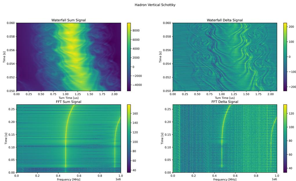
Figure 2: Waterfall diagram and frequency analysis of beam injection with the Libera Hadron.
