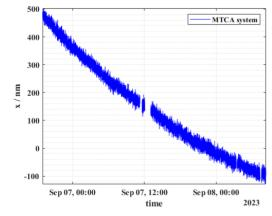
Figure 6: Horizontal position readings acquired from the SA data path with the MTCA based system and monitor constant  $K_x = 10$  mm. Gaps in the data indicate periods where the beam was lost.
