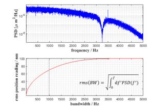
Figure 5: Horizontal power spectral density and closed orbit resolution as function of bandwidth, derived from the FA data path for the BPM with beam jitter cancellation. The monitor constant is  $K_x = 10$  mm.
