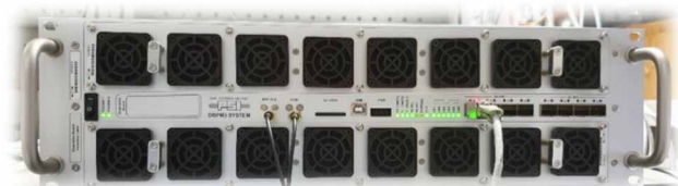
Figure 4: DBPM3 BPM electronics unit for SLS 2.0 with front-to-rear ventilation, redundant fans, and redundant power supply.
